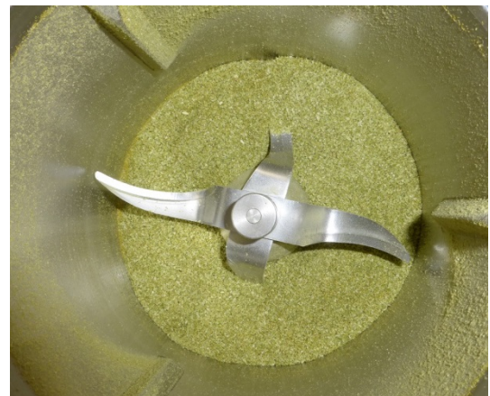
Fig. 2: Hops milled at 4,000 rpm, grinding time 15 seconds
