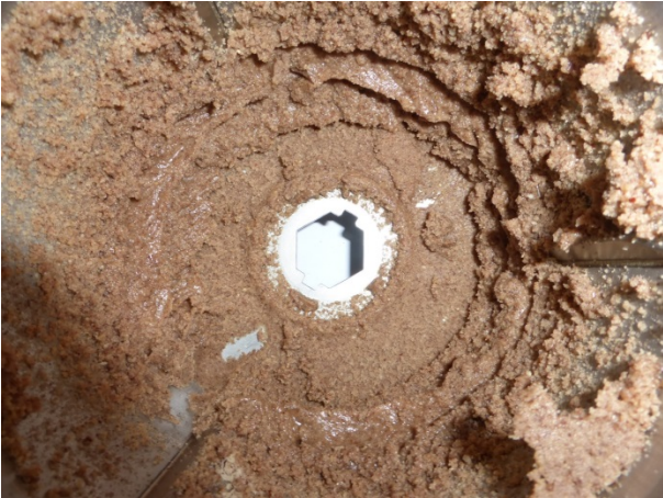
Fig. 6: Hazelnuts after 30 seconds grinding in the grinding vessel made of stainless steel
